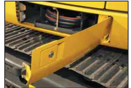
A large tool box provides plenty of space and room for the hose of the refuelling pump.
